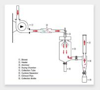
2. The self-priming peristaltic pump delivers the sample liquid from a container through a small diameter jet into the main chamber. At the same time an integral compressor pumps air into the outer tube of the jet which causes the liquid to emerge as a fine atomised spray into the drying chamber.
